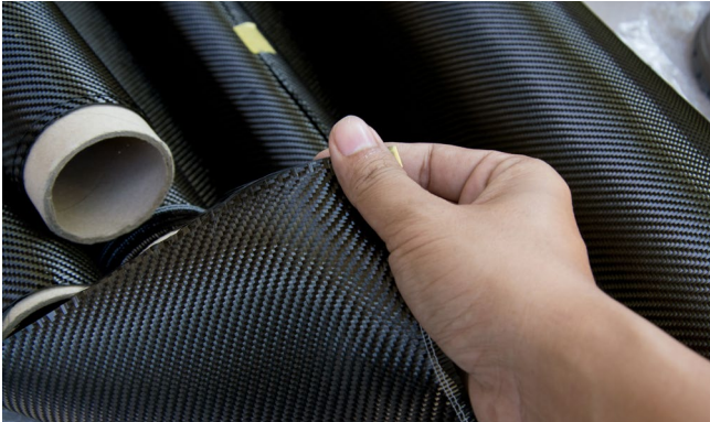
Carbon fibre composite raw material. Used widely in defence and aerospace products due to its exceptional strength-to-weight ratio.
