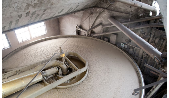
Pulping mill to prepare wood chips and plant fibres for paper production.
