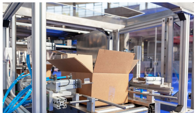
Automated cardboard box folding equipment to pre-assemble packaging.
