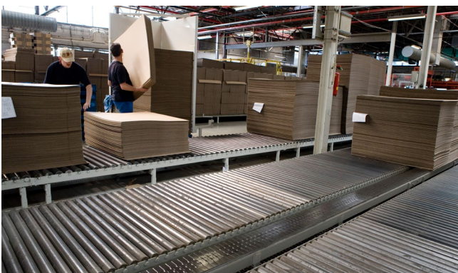
Laminated cardboard sheet production line with conveyor systems.
