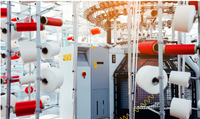
A circular weaving loom machine can create a seamless woven fabric tubes.
