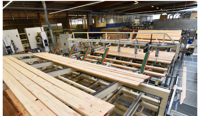
Laying up of processed timber to prepare for kiln drying process.
