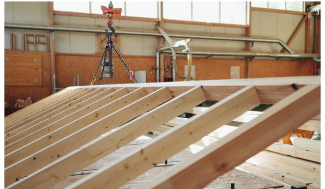
Pre-nailed framing for the construction industry to prepare for onsite installation.
