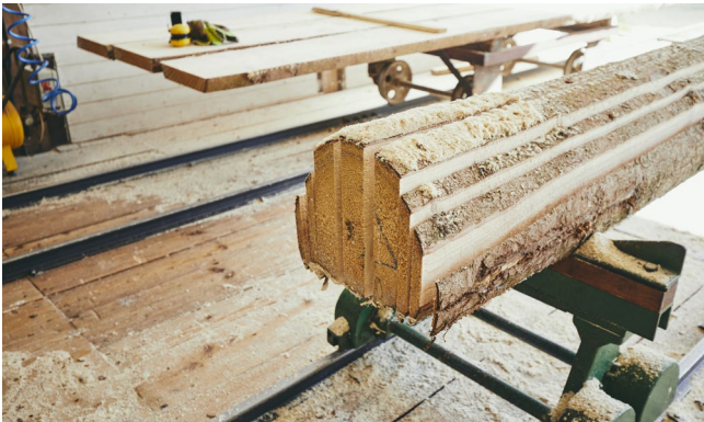
Example of a 'plain sawn' log to maximise use of material.
