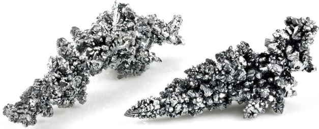
Vanadium, a naturally occurring element mined in Queensland. It is used to make long lasting batteries.
