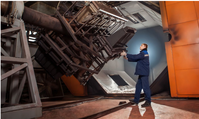
A production technician guiding a rotational molding arm into a heating chamber.
