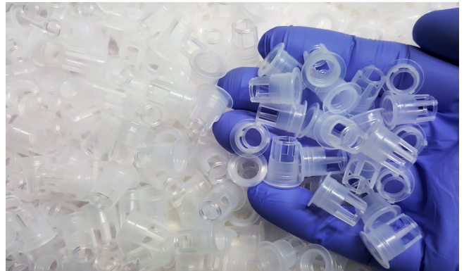
Small injection molded plastic parts in a recovery bin for collection and inspection.
